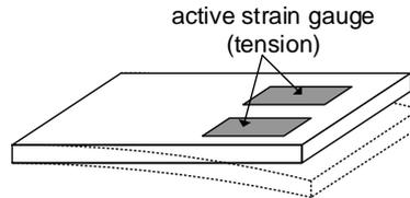
Figure 1: Metal strip with two active strain gauges.
