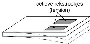
Figure 1: Metal strip with two active strain gauges.
