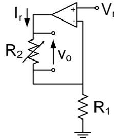
Figure 7: Temperature sensor.
