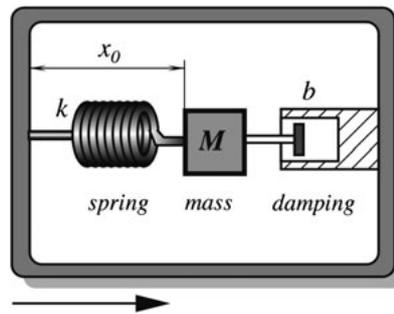
Figure 1: Mechanical model of an acceleration sensor.
