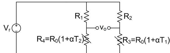
Figure 2: Electrical equivalent circuit of mass airflow sensor.
