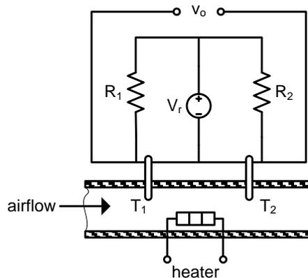
Figure 1: Mass airflow sensor.
