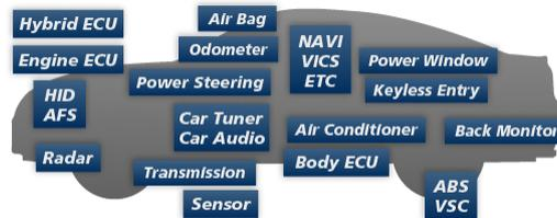
Figure 1: Applications of electronic control units (ECUs).
