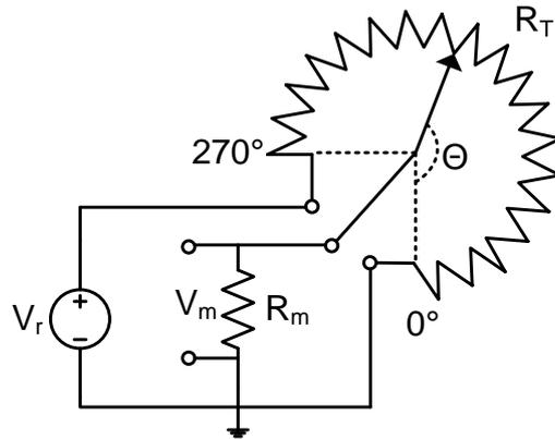
Figure 1: Throttle position sensor with processing circuit.
