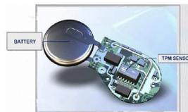
Figure 2: Tire-pressure sensor.
