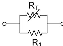
Figure 1: Linearisation of a silicon resistive detector.
