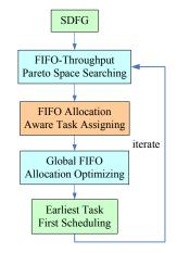
Fig. 3. The framework of the Iteration-based Task-FIFO Co-Scheduling Algorithm.
